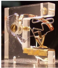
Copy of the first transistor by Shockley, Brattain
